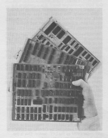
The board is addressed at CF00 and can be accessed directly from OS-65U basic as DEVICE 3 or DEVICE 8 with the input/output being routed to any port on the board. This routing is defined by the use of the program PRTSET.
