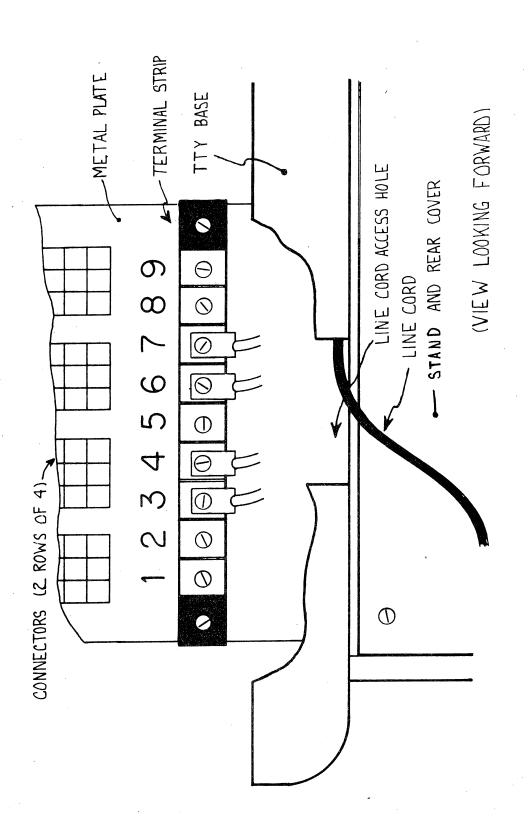
Diagram  $\mbox{\mbox{$\mbox{$\mbox{$\mbox{$\mu$}}$}}$  . Connecting to a Teletype
